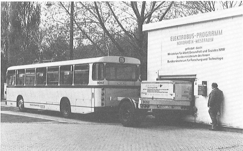
Fig. 2: Battery Powered Urban Bus supplied by Battery Changing
