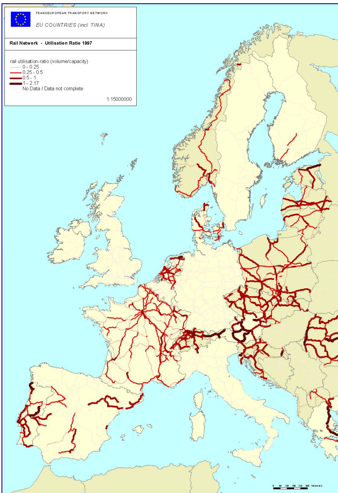
Figure 4: Utilisation of Rail Capacity on the Trans-European Rail Network (data from the DG TREN GISCO Database)
