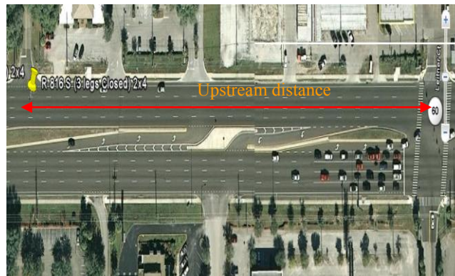
Figure 1: Upstream Distance Measure between Unsignalized and Signalized Intersections
