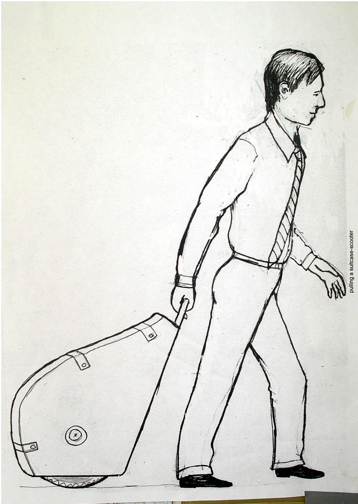
Fig (1). The wheels of the 'suitcase scooter" protrude slightly from the case. They give little friction when freewheeling as the wheels are about 300mm in diameter
