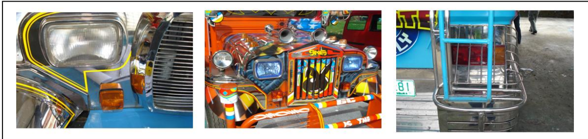
Figure 10 - Jeepney's Light and Light Signaling Devices
