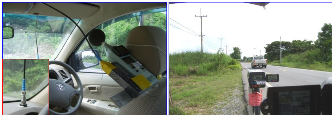
Figure 3 In-vehicle sound, vibration, and speed measurements
