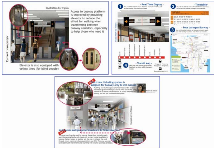
Figure 8 – Interchange Facility Improvement Graphics
