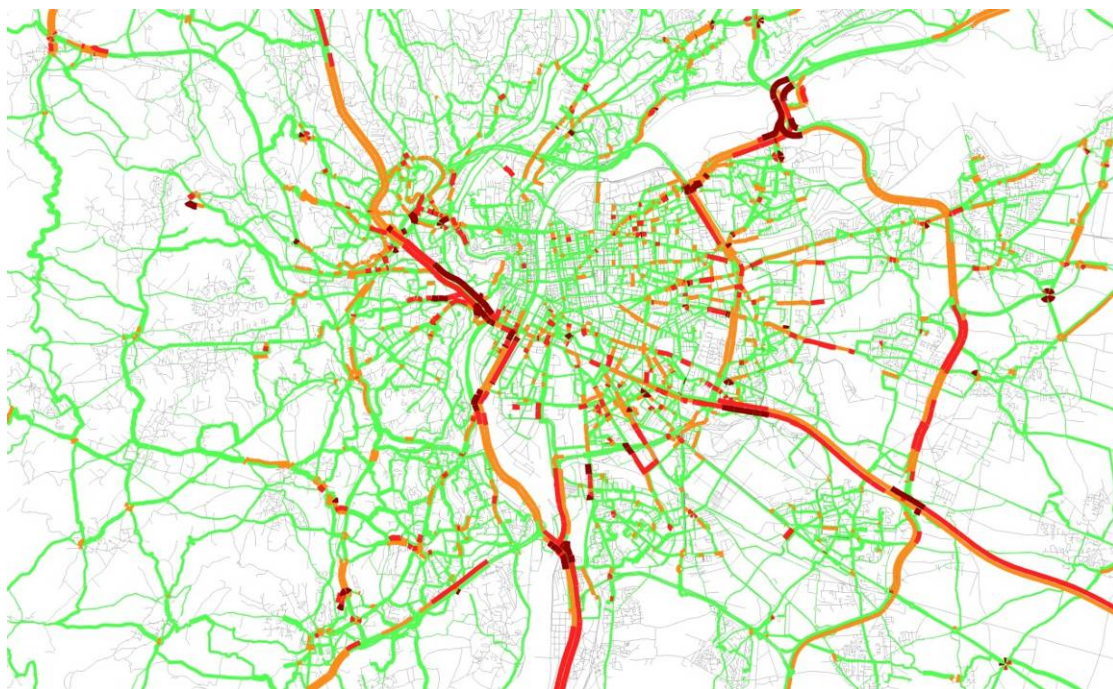
Figure 7 – Example of saturation rates on various road sections
