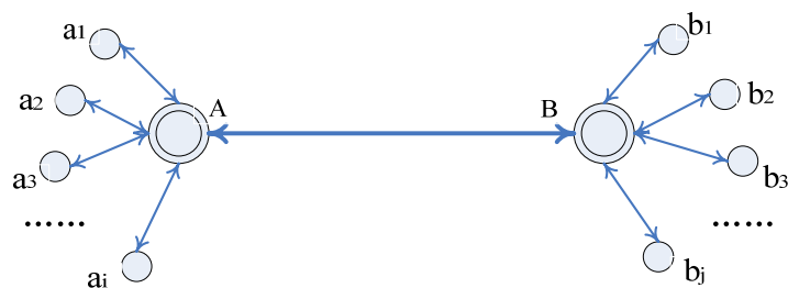
Figure 2 (b)-The "dog-bone" type of hub-spoke air network
