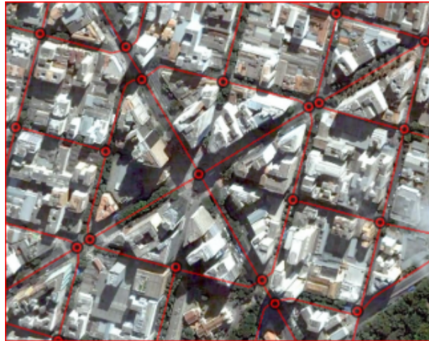
Figure 1: Network model of the transport system of Sete de Setembro Square (BH, Brazil)
