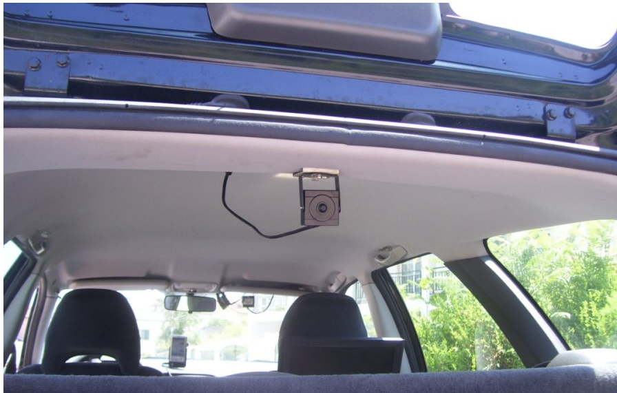
Figure 10 – Rear view camera
