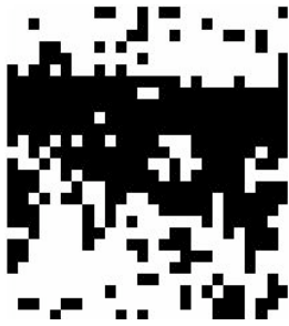
A: Texture Classified Image in Which White Squares Represent Ballast and Black Squares Represent Non-ballast Areas
