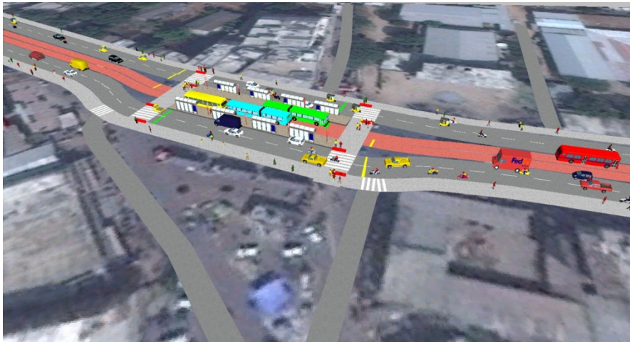
Figure 9: Simulation of one measure of case study 2: median bus lane and bus stop (Source: own graphic, based on simulation model VISSIM & google maps).
