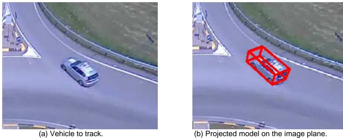
Figure 5: Example of expected result when the correct parallelepiped model is projected on to the image plane.
