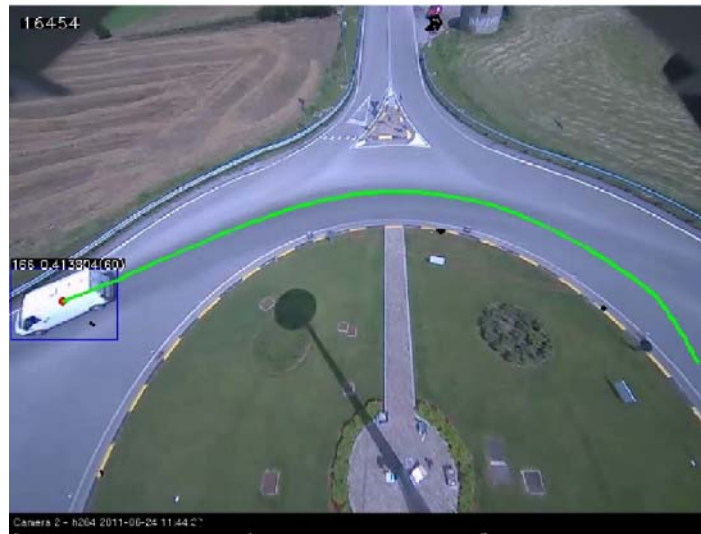
Figure 4: 2D vehicle trajectory extracted on the image plane using the algorithm in (Mussone et al., 2011).
