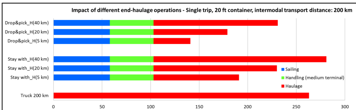
Figure 10 Impact of different end-haulage operations on cost competitiveness of intermodal IWT (at 200 km)
