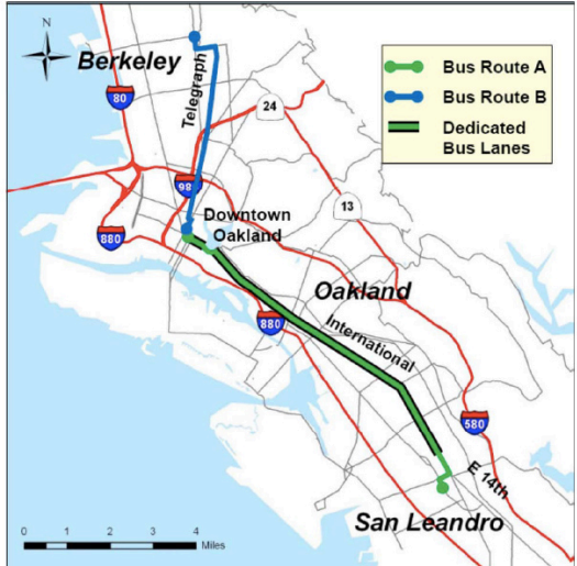
Figure 3: The Downtown Oakland-San Leandro Alternative plan for East Bay BRT. Source: AC Transit.
