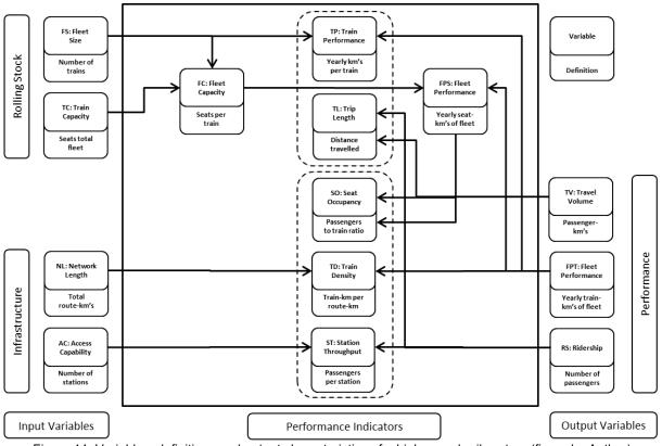
Figure 11: Variables, definitions and output characteristics of a high-speed rail system (figure by Author)
