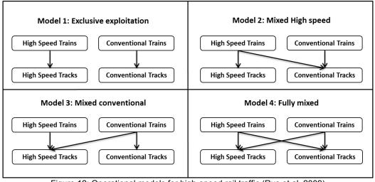
Figure 12: Operational models for high-speed rail traffic (Rus et al. 2009)
