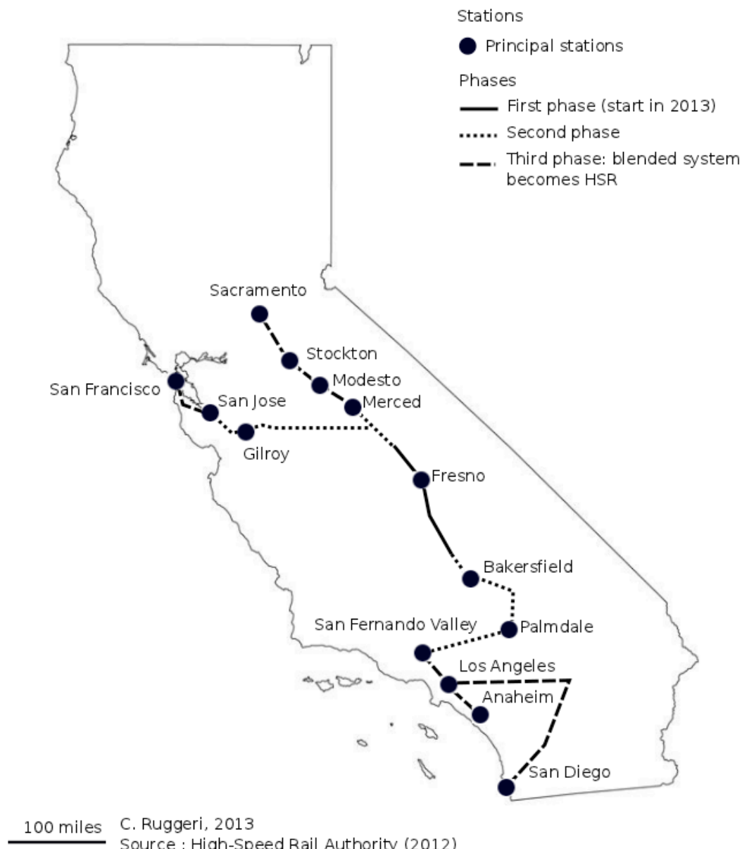
Figure 2 – Construction phases of the high-speed rail
