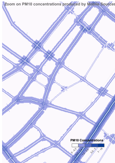
Figure 9 – Map: Model simplifications; Visualization of concentration value at intersections and Gauss distribution around a link.
