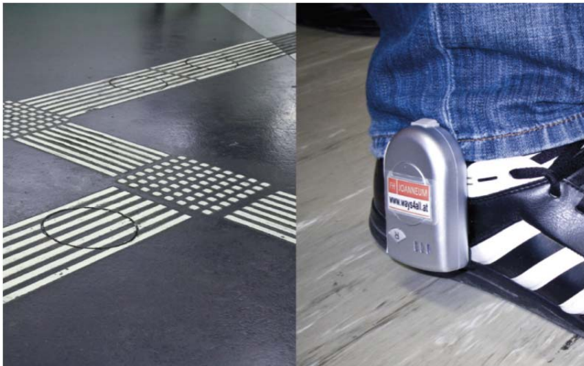
Figure 20: Ways4all – RFID chip – prototype of a receiver, photo © Wiener Linien, 2012
