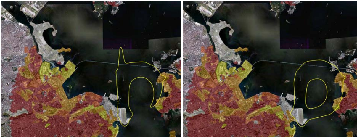
Figure 7: Areas with noise levels over 55 dB DNL: Runway 20 approaches, Current Scenario and Scenario 1
