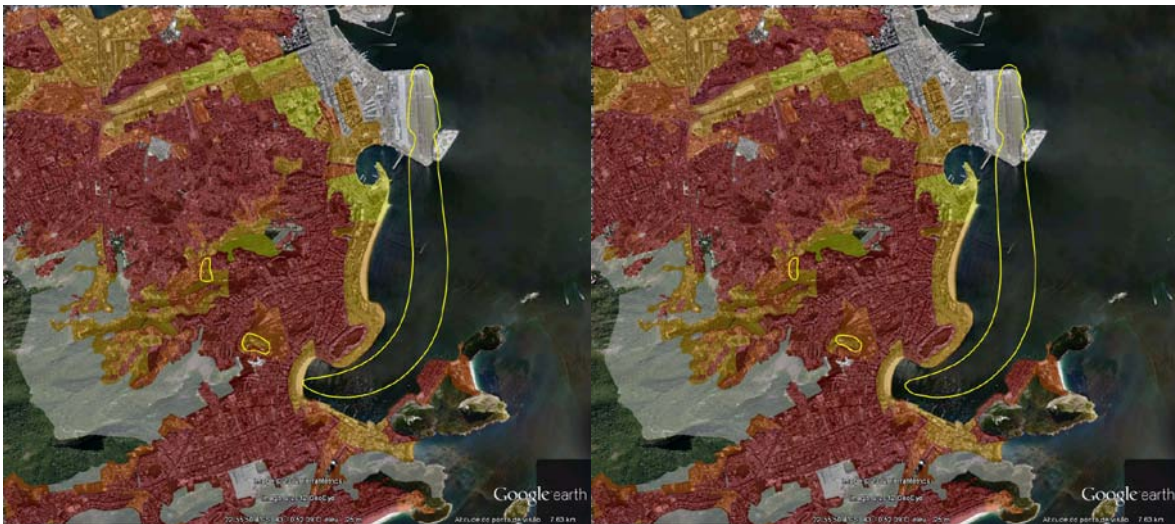
Figure 9: Areas with noise levels over 55 dB DNL: Runway 02 approaches, Current Scenario and Scenario 1
