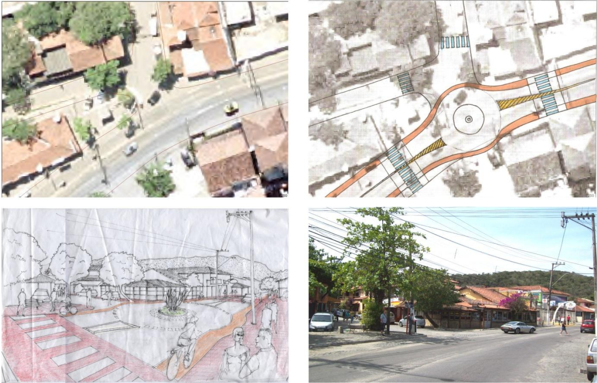
Figure 8 – Roundabout and pedestrian crossing leveled with the sidewalks
