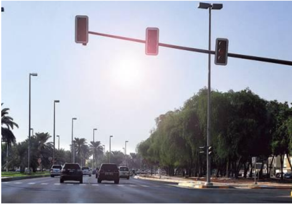
Figure 2 – Sun Glare Effects on Signal Lights (Source: Salama, 2010)
