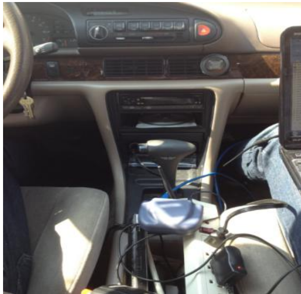
Figure 8 – The RFID receiver is inside a vehicle, however the antenna of which can be placed anywhere inside or outside the vehicle, depending on the connection availability
