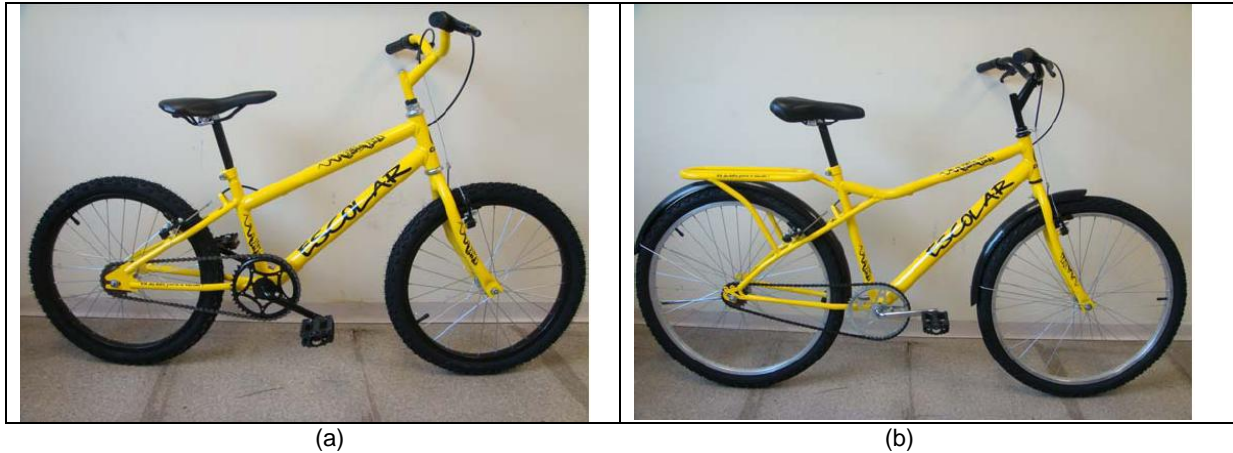
Figure 1 - 20-inch (a) and 26-inch (b) strengthened bicycles for school transport.
