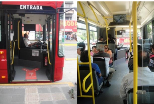
Figure 1i. Low Floor Entry and Bus Interior
