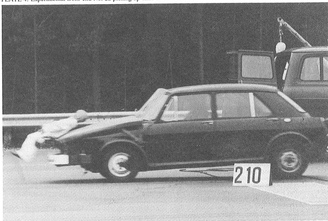
PLATE 4: Experimental front-end No. 2a picking up child at 16 km/h.
